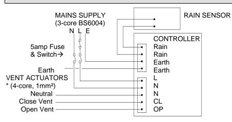
\* 3-core cable required if Vent Actuator does not require Earth (double-insulated)
