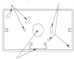
Cable entry/exit points (punch holes through box only where required). Use cable-clamping bar in best position and tighten the 2 clamp screws.
